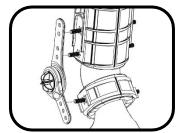
Manipulate hinge arms to place over appropriate bolts at upper and lower braces for proper fit.
