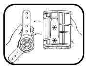
Remove hinge arms from uppera and lower cylinder braces.
