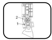
Once in place, **tighten lower hinge arms FIRST** (to ensure alignment) then geared hinges.
