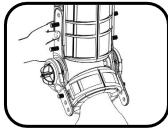
Be sure the hinge arms are properly positioned within preset slots before securing in place with wing nuts.
